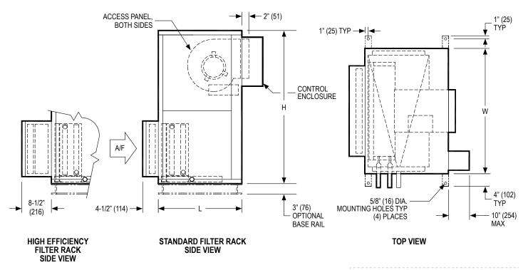
NOTES: Dimensions in parentheses are in millimeters (mm). See table below for dimensional references. Provide sufficient clearance to permit access to controls and comply with applicable codes and ordinances. Base rail is optional on the base unit. Base rails must be used with mixing box. Electric heaters are only available in fan arrangement 3.
